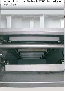
Each filter box is automatically cleaned during normal conveyor operation. Coolant flow and optimal filtration is assured, as the design of the Turbo MS500 allows the number of filter boxes used to be matched to the requirements of the machine tools maximum flow rate.
